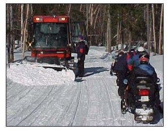
necessary corrections to the trail, **Photo 3.2** Stop only where there is good sight distance then get underway again. If the stop is anticipated to take a longer period of time, consider placing warning devices, like what are shown in Figure 3.1, on the trail to warn snowmobiles of the groomer's presence.
